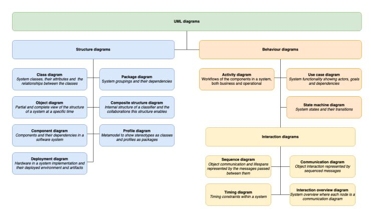
Figure 6 UML diagram types [16].
